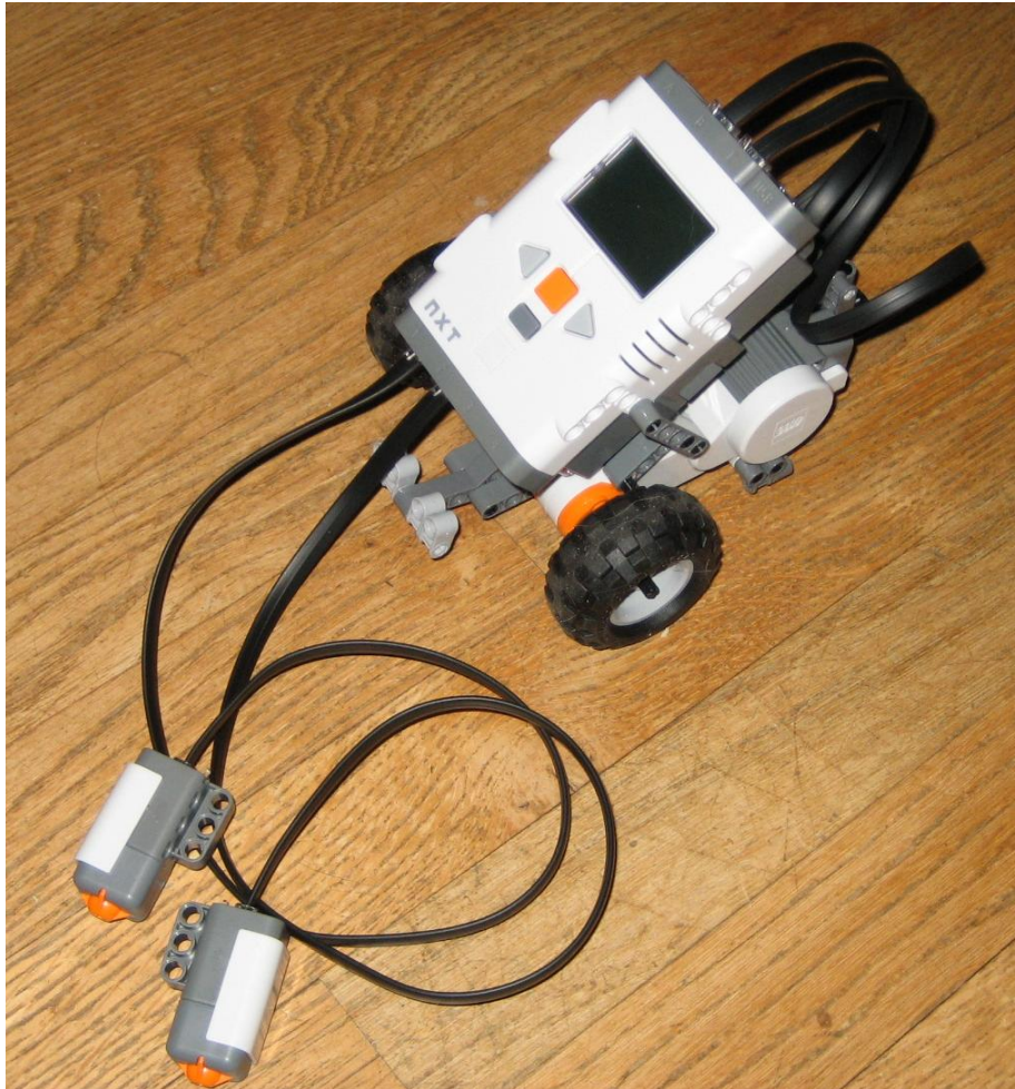
Picture of Rover with 2 touch sensors connected
